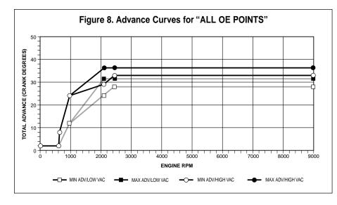
the dial-back timing light. Connect the dial-back timing light to the front cylinder. Set the HI-4 advance trimpot full clockwise for maximum advance. Run the engine at 2,500 RPM. Adjust HI-4 position until TDC timing mark is centered in the observation hole. You will now have the amount of advance you dialed into the timing light.
