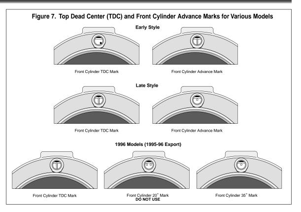
Run the engine at 2,400 to 2,500 RPM. Adjust HI-4 position until advance timing mark is centered in the observation hole. Tighten the standoffs and verify that timing has not shifted.
