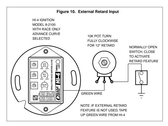
retard feature, the green wire is connected to a 10K pot (potentiometer), which in turn is connected via a switch to ground as shown in Figure 10. The 10K pot is used to set the amount of retard. When the switch is closed, the retard feature is activated. A sealed MIL-SPEC 10K potentiometer (Clarostat RV4LAYSA103A) with locking shaft is available from Newark Electronics (312-638-7652).
