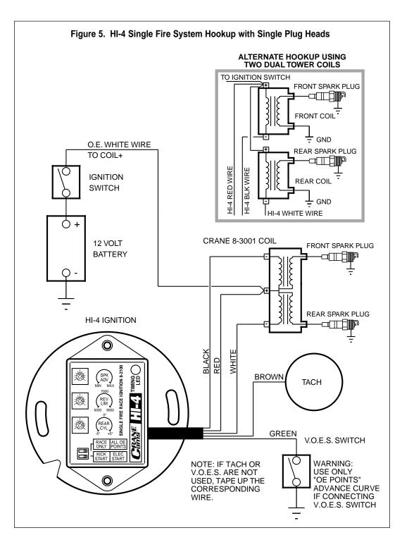
Race Only Applications. When using the "RACE ONLY" advance curve, vacuum advance is not supported. Tape up the unused green vacuum switch wire from the HI-4 or refer to the section: "EXTER-NAL RETARD INPUT CAPA-BILITY FOR RACE ONLY ADVANCE CURVE" later in these instructions.
